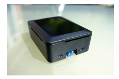
The universal input module is a simple device to integrate third party devices to one another. Operating from low voltage USB supplies, it can be configured via Wi-Fi or ethernet connections. The Camect firmware allows you to switch Camect from normal to home mode via a voltage free input - from an intruder panel, access control system, NVR etc
